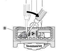
4. Turn the adjustment bolt on the pedal to adjust the spring tension to the strongest setting.
